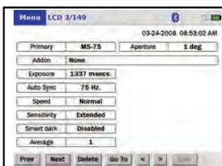
The patented Auto Sync® feature takes the worry out of accurately measuring high intensity, fast refreshing sources such as LCD's, PDP's, DLP Projectors, etc. by adjusting the detector exposure time to the source refresh rate. When enabled Auto Sync® insures that entire pulses are captured, improving the accuracy and repeatability of the measurements. The Sync rate of the source is displayed once a measurement is completed.
