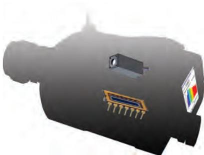
The PR-680 and 680L SpectraDuo<sup>®</sup> are the first and only instruments to contain a fast-scanning 256 detector element spectroradiometer and an ultra-sensitive, low noise Photo Multiplier Tube based filter photometer in one. Available operating Modes are: 1) As a fast scanning spectroradiometer 2) As a highly sensitive photometer or 3) Auto Select Mode which automatically chooses the detector based on the available signal.
